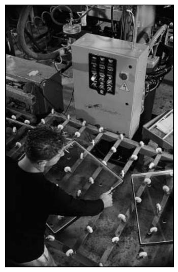
Operating the new system simply required the operator to adjust the air pressure to maintain bead consistency from one size to the next after he's switched heads. It's a simple chore. "There's no waiting with the new pump, I don't have to bleed the system. It 's just so much easier to operate," he says.
