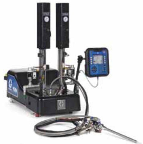
Figure 6 The Graco PR70 with accumulators can be used for lower output, spiral wound, membrane adhesive bead applications with higher-viscosity materials. Handheld gun shown with disposable static mixer
