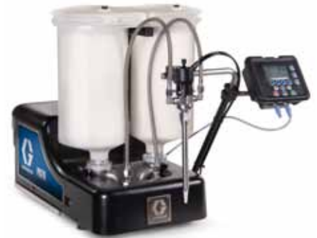
Figure 5 The Graco PR70 Meter, Mix and Dispense unit is a bench top system for manually dispensing smaller shots, end caps or hollow fiber potting applications. Fixed mount dispense valve shown with disposable static mixer.
